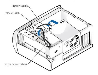
When you rotate the power supply back into the computer, gently lift the and hold the drive cables out of the way. Rotate the power supply into position until its release latch clicks. Lay the drive power cables along the top of the latch.
